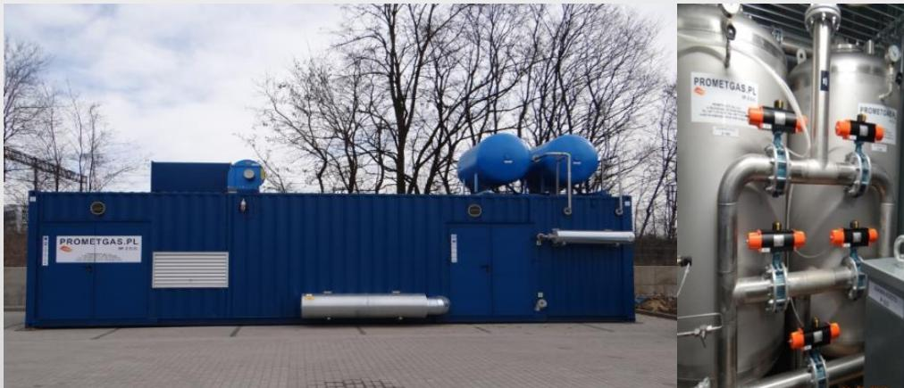
Air separation mobile pilot plant
