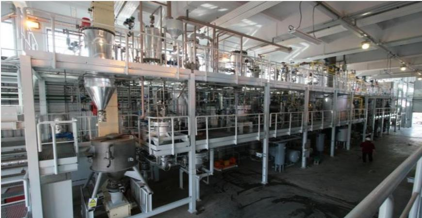
Pressurized CFB oxy combustion pilot reactor (0,2 MW)
