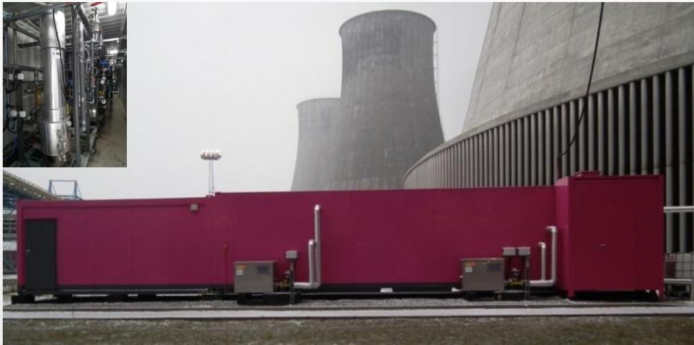
VPSA CO<sub>2</sub> capture mobile pilot plant
